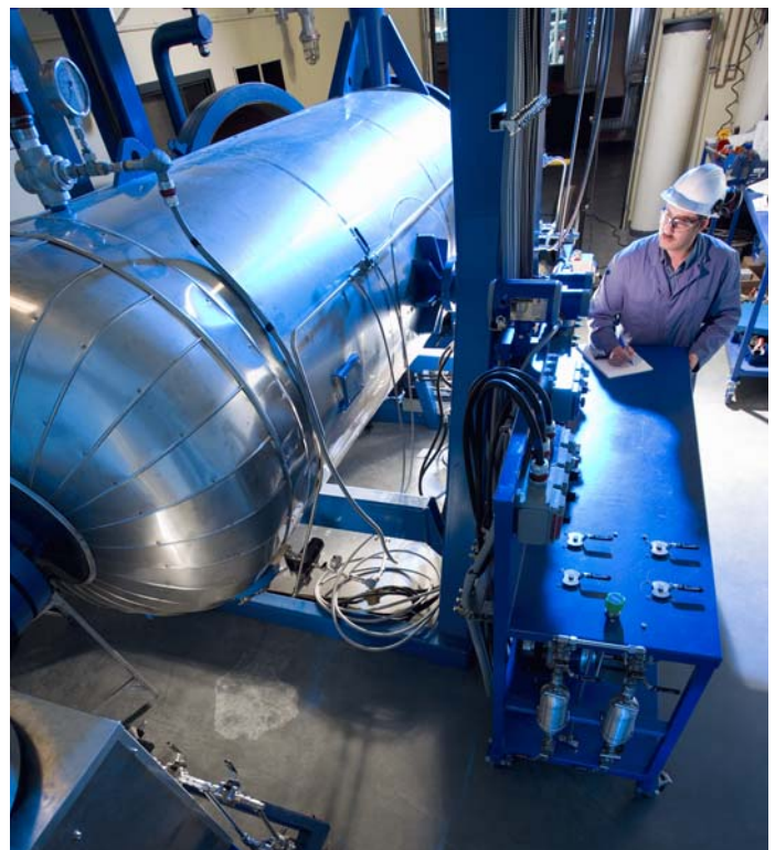
SRC Senior Research Engineer Kelly Knorr at work commissioning a new 3D scaled physical model to be used for testing different vapour extraction solvents and strategies.
