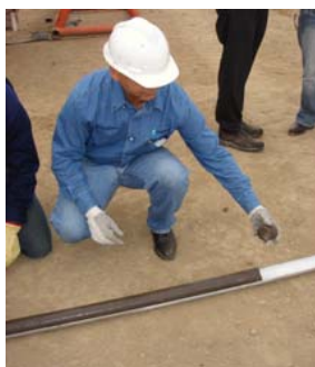
Rock samples from potential storage sites are used to analyze the rocks and the properties that affect the safety and security of storage.
